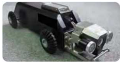
TV camera describing the inside condition of pipelines
