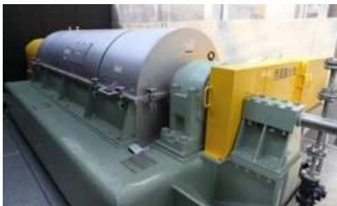
Two-agent sludge conditioning centrifugal dewatering device
