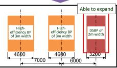
Down sized dewatering device works for limited space
