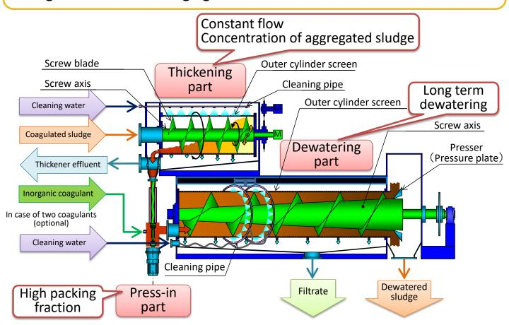
Scope of application: thickened sludge including mixed sludge, anaerobic digested sludge, excess sludge, etc.
