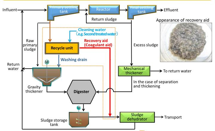
Scope of application: WWTP with a primary settling tank : Scope of application
