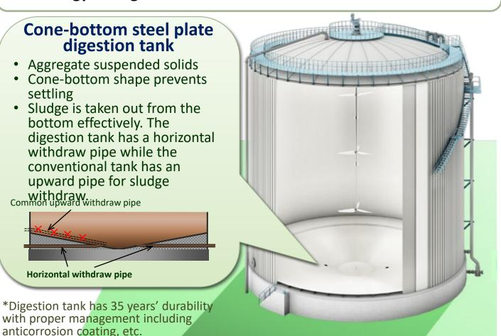
Target: primary/excess sludge, human waste, septic tank sludge, and biomass such as food waste
