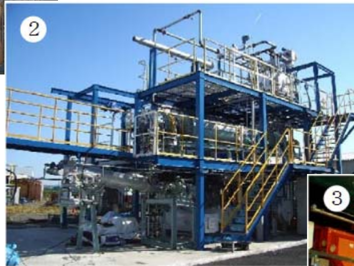
② Development of sewage sludge fuelization technology adaptable to coal-fired power plant
