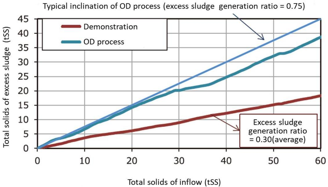
Figure 2: Comparison of total solids of excess sludge between demonstration and OD process
