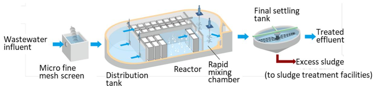
Figure 1: Image of the demonstration technology
