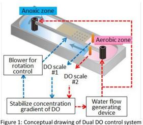
Figure 1: Conceptual drawing of Dual DO control system in OD process
